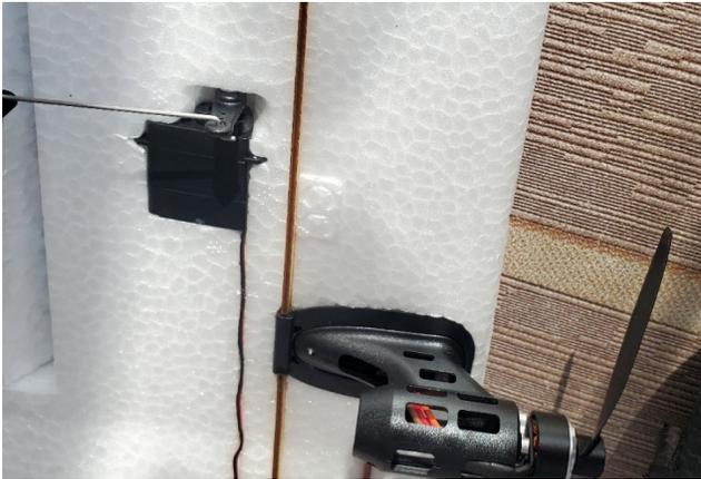
The plane is equipped with a full-flying T elevator and twin ailerons (each with a servo). The motors are held in place by pylons screwed into hardpoints in the foam wing. The wing is one piece and removeable.
