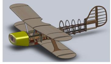
106"x18" wings are going to be beautiful in the air! I've already CNChotwire cut the wings and a rough cowl and later in the month I'll start laser cutting the fuselage parts. I acquired the landing gear as well as the wing and stab tubes to make the wings and stabs removeable. The wing center sections will be permanently attached to the fuselage. Stay tunned!
