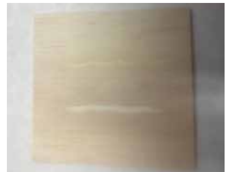
And here's the final piece after a light sanding. The mix is just about invisible, and is harder and stronger than just the spackle alone.
