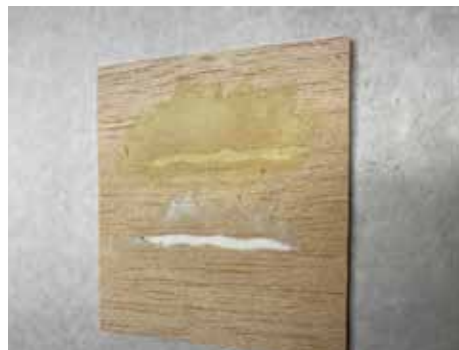
Here's our sample gaps, filled and the excess filler mix scraped off. The white area is just the spackle... the cream colored area is the mix.
