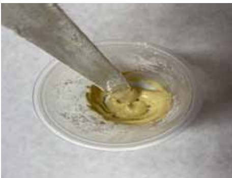
Mix the Durham's putty with water first, to a consistency about like yogurt. Then add the DAP lightweight spackle.
